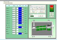
This system includes user-friendly control software that provides a graphical representation of all system components, zone temperature settings, actual temperatures, and belt-speed. Security password protection prevents unauthorized changes ;Pre-program the weekly operating schedule is available
