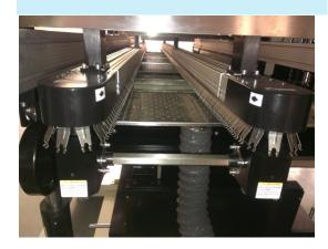
Conveyor angle is adjustable from  $4^{\circ}$  -  $7^{\circ}$  and nominal speed setting is variable from 0.5 - 2.2 m/min (20" - 87"/min) for maximized throughput.
