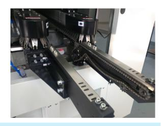
An optional center PCB support rail can be added to maintain planarity and to prevent sagging of oversize boards through the wave module.
